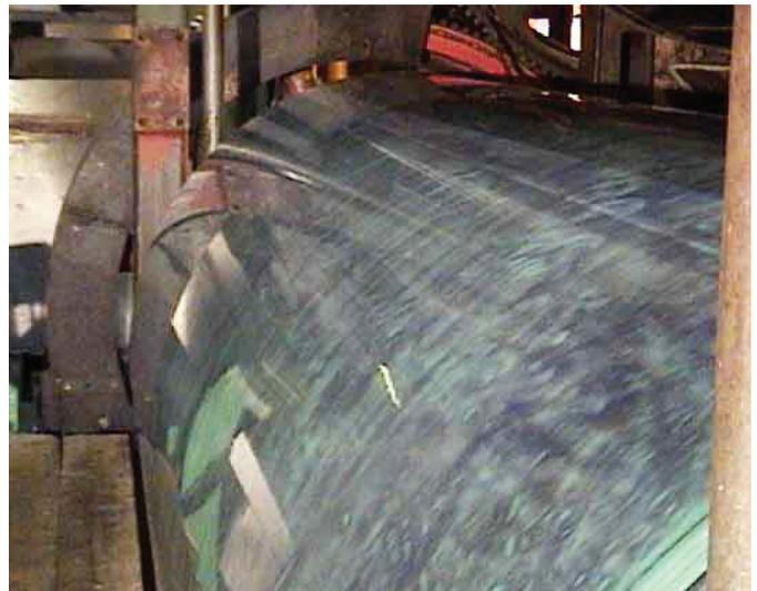
The roll cover is bonded to the dryer by injecting the adhesive under the end of the sleeve. It is then cured at maximum temperature.
