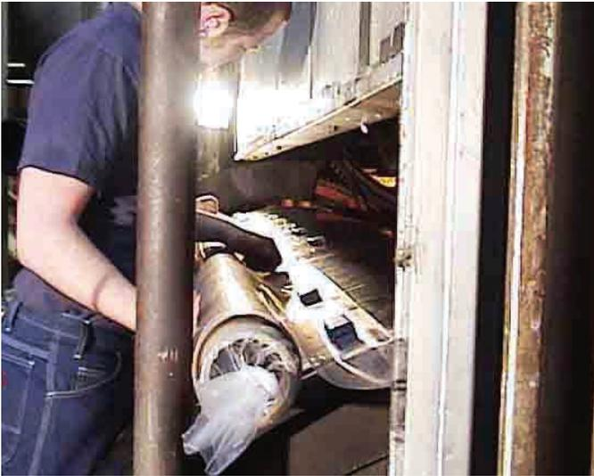
The dryer's surface is first cleaned to provide a good surface for bonding. The heat shrinkable film is then rolled around the dryer and the sealer is put in place. The film is then sealed to complete the tube. The seal's strength is as strong as the material itself.
